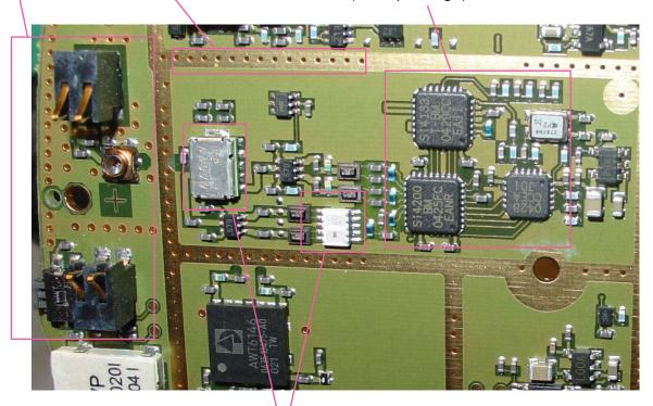
Electromechanical (acoustic wave) bandpass filters
