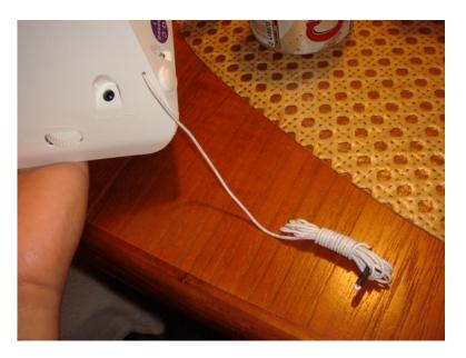
This is your antenna. It can be unrolled to clear interference from the electronics and to get better reception without having to move the clock unit itself.
