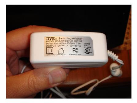
Power adapter is OEM logo'd. Allows for DVE to pay for the UL registration, etc. etc.
